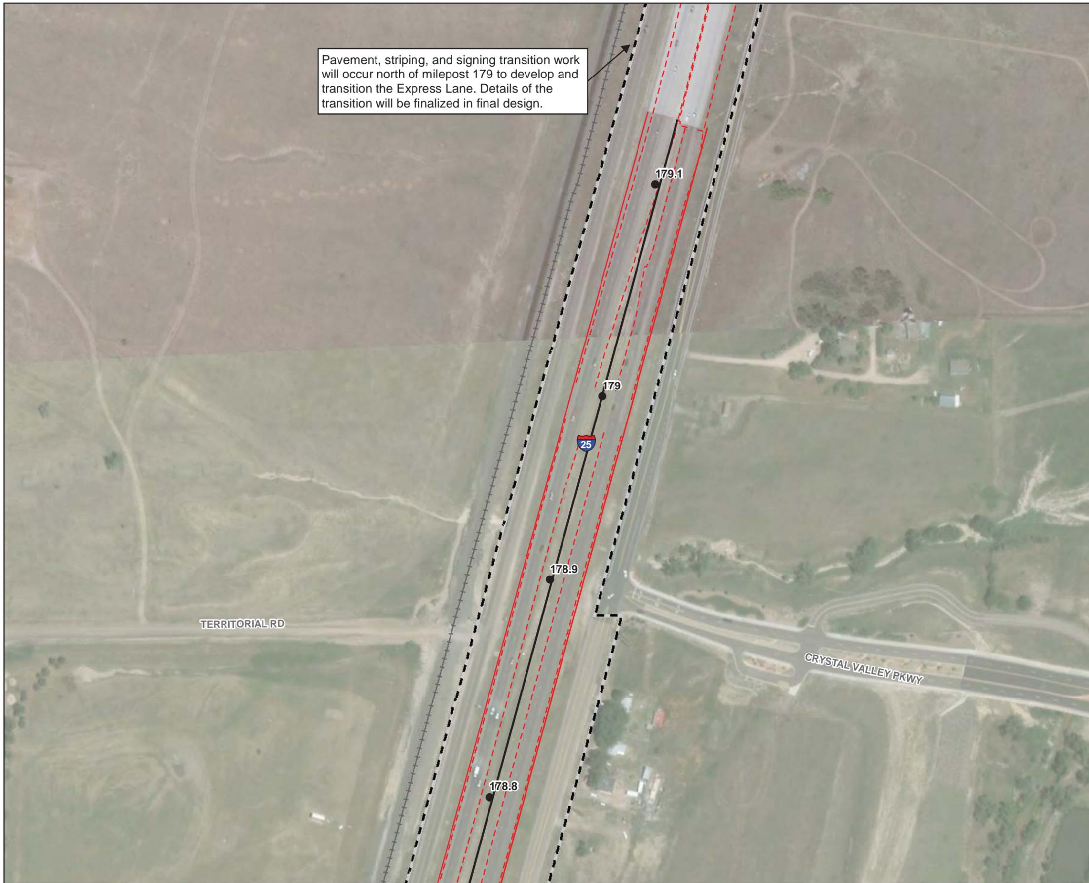
Pavement, striping, and signing transition work will occur north of milepost 179 to develop and transition the Express Lane. Details of the transition will be finalized in final design.
